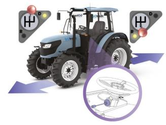
The GEAR PLUS series device is designed for tractors equipped with electric or electrohydraulic reverser. The device controls the tractor's forward and reverse drive, in one gear selected by the user. In such tractors, the change of travel direction is carried out by electronically controlled switches. Only in tractors with this equipment is it possible to install the GEAR PLUS series and properly use the device's functions.
