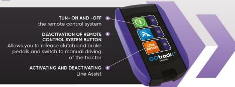
Turn -on and -off is possible only by using smart panel, which is mounted on tractor's cocpit or dashborad
